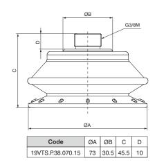
Round bellows suction cup made of polyurethane, suited for movement of pieces of various size and shape and where level compensation is necessary, such as when withdrawing from loaders. The big advantage of this suction cup is that the material it is made of--polyurethane--lasts longer than other materials, has optimum wear resistance, good flexibility and optimum tensile strength. Polyurethane suction cups are mark resistant.
