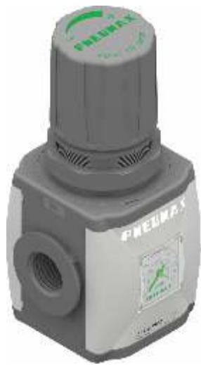
Example : T173BRMC : size 3, Regulator including gauge with Technopolymer threads, G1/2" connections, 0 to 8 bar adjusting range
