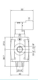
Example: T171BVEB2: size 1, Electric shut-off valve, with M2 Pilot without coil, Technopolymer threads, G1/4" connections
